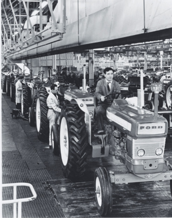
END OF THE LINE – AFTER FINAL INSPECTION TRACTORS ARE DRIVEN OFF THE PRODUCTION LINE TO AN 800 CAPACITY PARKING AREA TO AWAIT DISPATCH.
